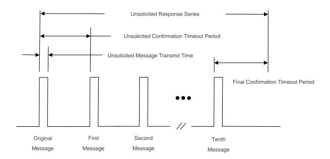
After the original message in sent, the outstation waits two seconds for the master confirmation, this time is shown as the *Unsolicited Confirmation Timeout Period* in the figure. If the outstation does not receive any confirmation from the master, then the outstation replies the original message in a serie of ten messages.
